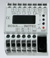
INOTEC Battery-Control-System for monitoring and logging block voltage and temperature of each battery block. Allows early detection and reporting of defective battery blocks. Automatic shutdown of the load and interruption of duration tests due to block failures to protect against destruction of the entire battery.
