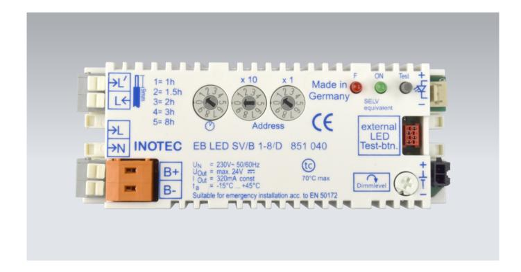
LED-driver with integrated individual lamp monitoring for non-maintained, maintained and switched-maintained lighting. With integrated charging technology and freely selectable nominal operating time of 1h, 1,5h, 2h, 3h or 8h with INOTEC SV/B- function control to connect to a central monitoring device BNS-MTB according to DIN EN 50172, DIN VDE 0100-718 and DIN VDE V 0108-100-1.
