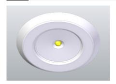
LED safety luminaire with optimised light distribution for the illumination of areas with high mounting heights. Housing made of powder-coated aluminium for installation in Ø 68mm ceiling cutout. Incl. 4-chip LED illuminant for maximum safety.
